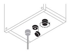
**Step 2** Connect camera system to control box by plugging in both connectors of braided cable coming from camera. Connectors go into either socket and should snap firmly in place.
