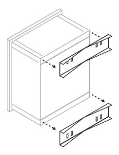
**Step 2** Attach mounting feet to back of control box using same screws and drill with Phillips #2 bit.
