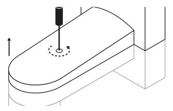
**Step 4** Push camera up into pendant housing and rotate a quarter turn until it snaps into place, aligning with screw holes...
