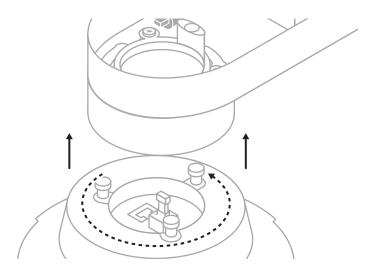
**Step 6** Secure camera to pendant housing by tightening screws using T30 Torx screwdriver.
