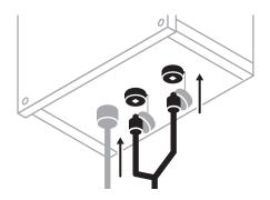
**Step 3** Twist protective plug caps on connectors up into bottom of control box. This will create a watertight seal.
