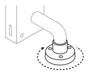
**Step 4** Secure pendant to top of camera by tightening previously removed screws from Step 1 using Phillips #3 screwdriver.
