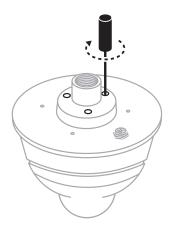
**Step 5** Secure camera to ceiling mount by hand-twisting pendant onto ceiling mount clockwise.
