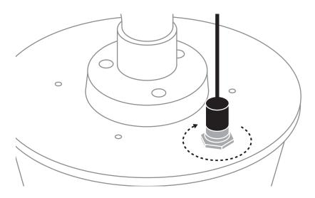
**Step 4** Plug other end of 110V cable into power outlet. Cable end will light up green when supplied with power.
