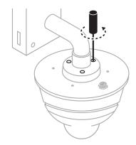
**Step 2** Loosen screw on inside of pendant using T20 Torx screwdriver (not included).
