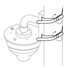
**Step 3** Trim steel straps to desired length using tin snips (not included).
