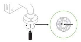
**Step 3** Remove pendant from mount by hand-twisting pendant clockwise.
