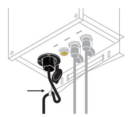
**Step 3** Plug other side of cable into a 110V power outlet.
