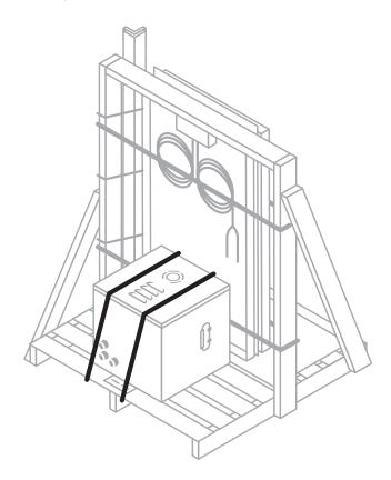
**Step 4** Place one battery on each side of the battery enclosure and secure them with the two 80" buckle straps going vertically across the tops.
