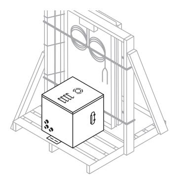
**Step 3** Using the two 105" buckle straps, secure the battery enclosure to the pallet with the straps going vertically across the top.
