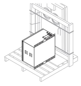
**Step 3** Place two batteries on each side of the battery enclosure and secure them with the two 110" buckle straps going vertically across the tops.
