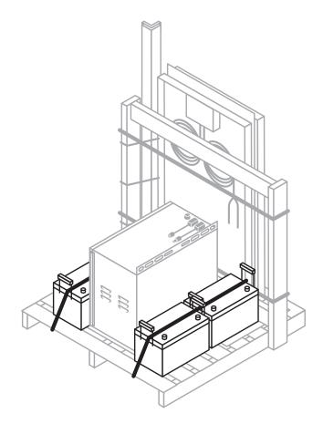
**Step 4** Secure the battery enclosure and batteries with two 145" buckle straps going horizontally across the tops. Thread the straps through the mounting slots on the battery enclosure for extra security.
