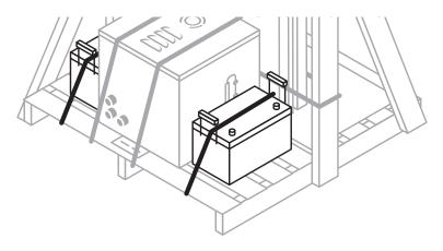
**Step 5** Secure the battery enclosure and batteries with the 145" buckle strap going horizontally across the tops.
